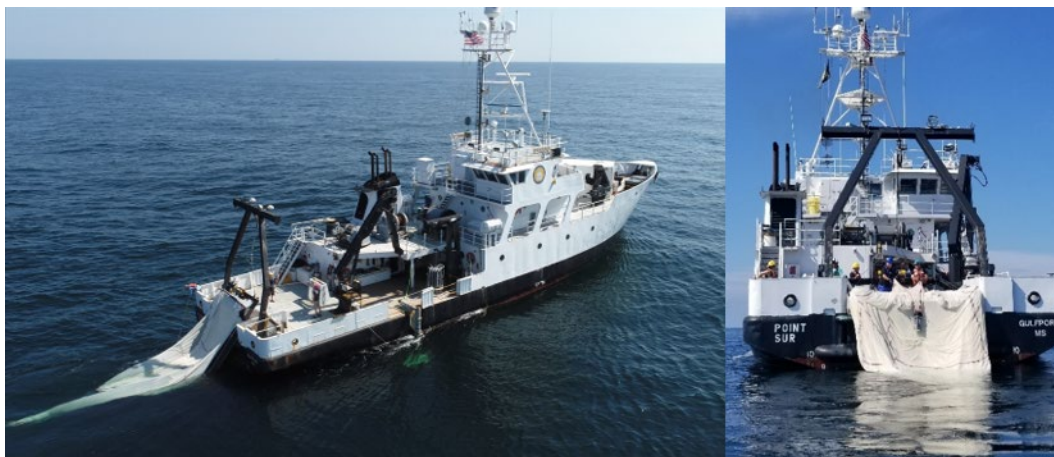
Figure 3. 10-m 2 MOCNESS unit being retrieved (left) and codends being retrieved (right) on the R/V Point Sur during DEEPEND cruise DP06. Photo: DEEPEND 2018/Danté Fenolio.
