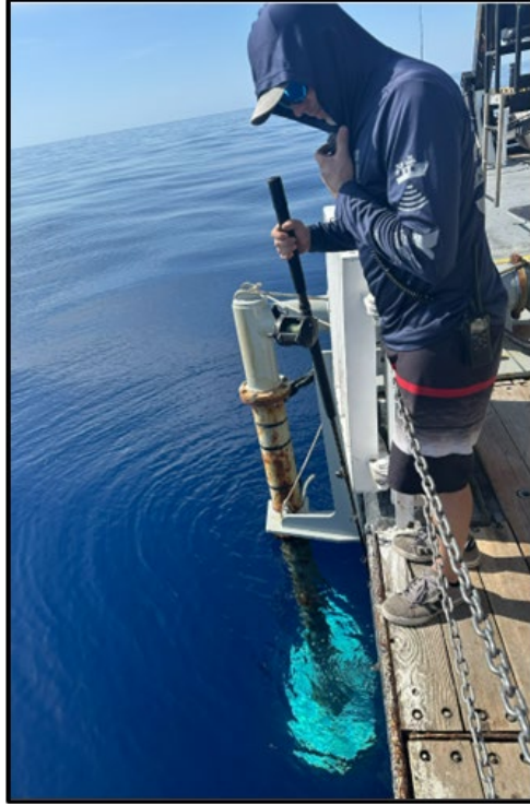
Figure 5. Kevin Boswell calibrating an echosounder.
